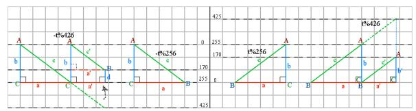
If you understand the image you can se that in the reverse t, a new height is made "d" wich is just the remaining of 255-170 wich is 85. This height "d" isnt relly a height itself but the "b" height of another sawthoot wave at its side.
