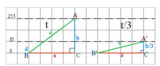
But we need to remember that "t" is an infinite diagonal line that is wrapped around and output of 255, so the hypotenuse "c'" will continue until it reaches the 255 output becoming the real "t/3", while maintaining the same angles as the false one.
